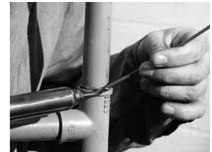
Figure 9-18. This welder blows heated air to join thermoplastics. (Laramy Products Co., Inc.)
