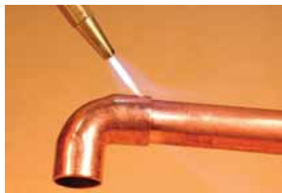
Figure 9-15. When the flux becomes liquid, shift the cone of the flame to the fitting.
